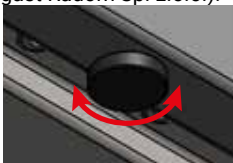
Figure 4. Leveling of the device
