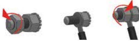
Figure 5. Connection of the device to an installation equalizing electrical potentials.
